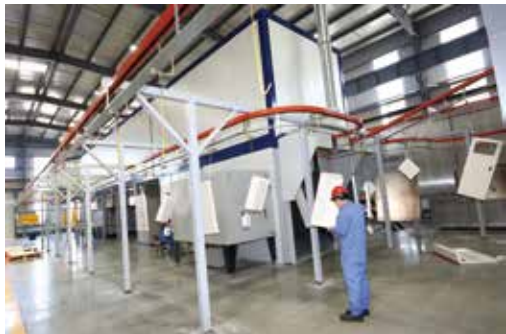
Automatic powder coating lines
